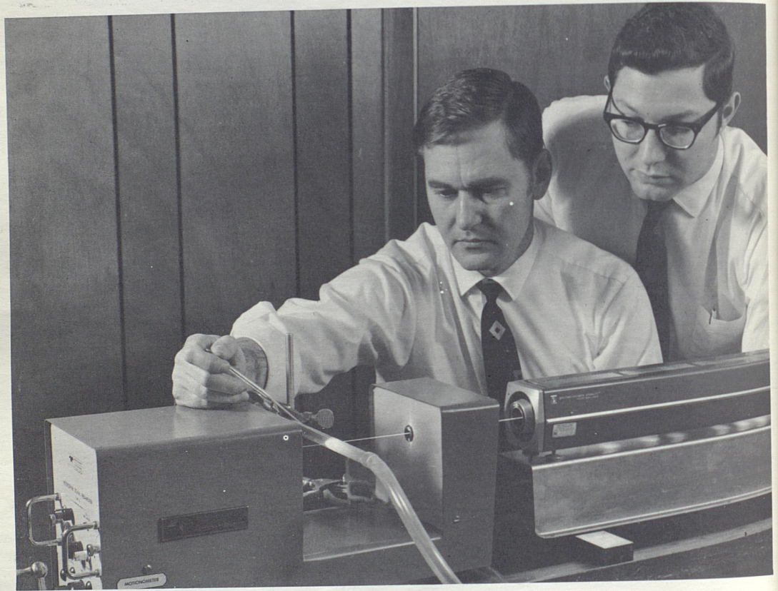
Dr. James F. Lafferty, acting director of the Wenner-Gren Laboratory (left) and Dr. C. F. Knapp, assistant professor of Mechanical Engineering, use a laser doppler velocimeter to study the fluid mechanics of the circulatory system.
