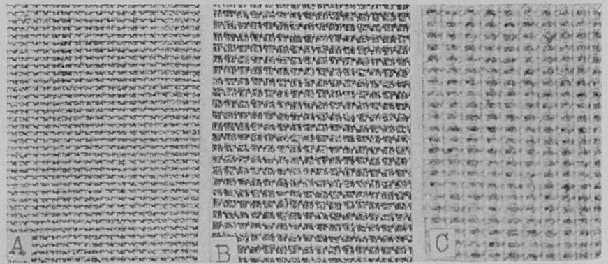
FIGURE 8. The wise purchaser examines the back of the floor covering. The closeness of the weave has an important relation to its wear. Each square in the weave represents a tuft. The number of tufts per square inch varies according to the type of weave and quality. Variations in tufts per square inch of highest and lowest grade Wilton, Brussels, Axminster and Velvet are given in the text.
