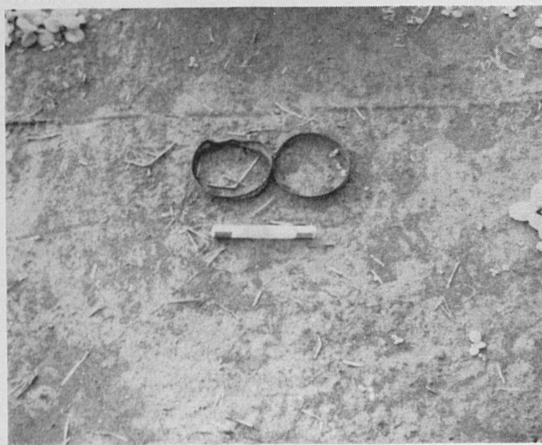
Fig. 2.— This plot received 1\frac{1}{2} pounds per square yard of calcium cyanamide in the fall but did not receive superphosphate. Note that no plants were produced. The circles are 7-inch cylinders driven into the ground. Water was percolated through them to determine if toxic materials from the cyanamide could be leached from the soil. Unless superphosphate was present, this leaching was not successful.
