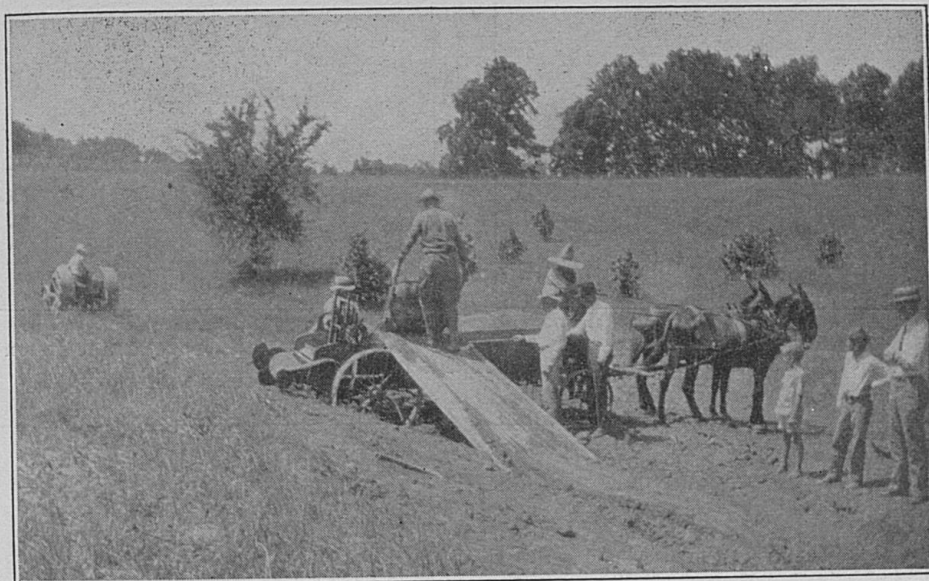
Loading marl with portable chute and tractor.
