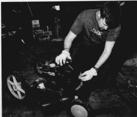
Brian Luck, an agricultural engineering senior, changes a spark plug on a lawn mower yesterday. The school's pre-professional group will continue to work through tomorrow.
