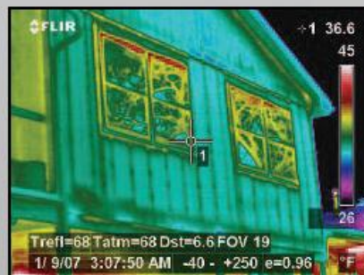
Under controlled temperature conditions when a thermographic camera focuses on a part of a building, it can reveal materials inside walls like old doors, windows, studs, corner posts, joists, and even nails.
