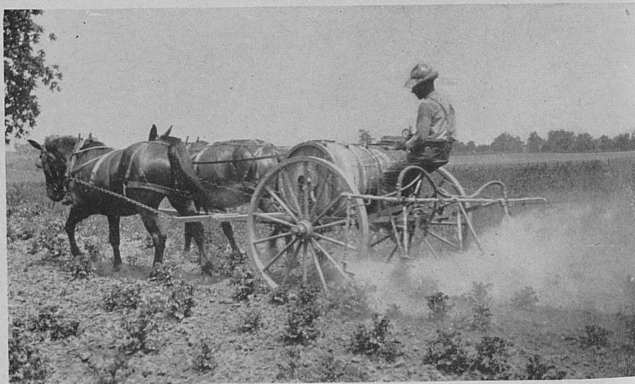
FIGURE 8. A traction-driven sprayer.
