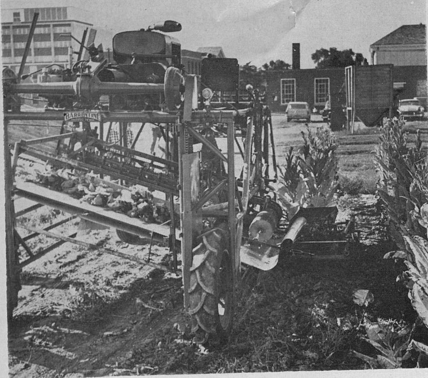
Rear view of the tobacco harvester (pilot model). Tobacco plants come from the right front, are cut, conveyed to position of cylinder in bottom foreground, speared automatically, and then transferred to tobacco stick. The loaded sticks are transferred to an accompanying wagon by the broad canvas belt on which loaded sticks are now lying.
