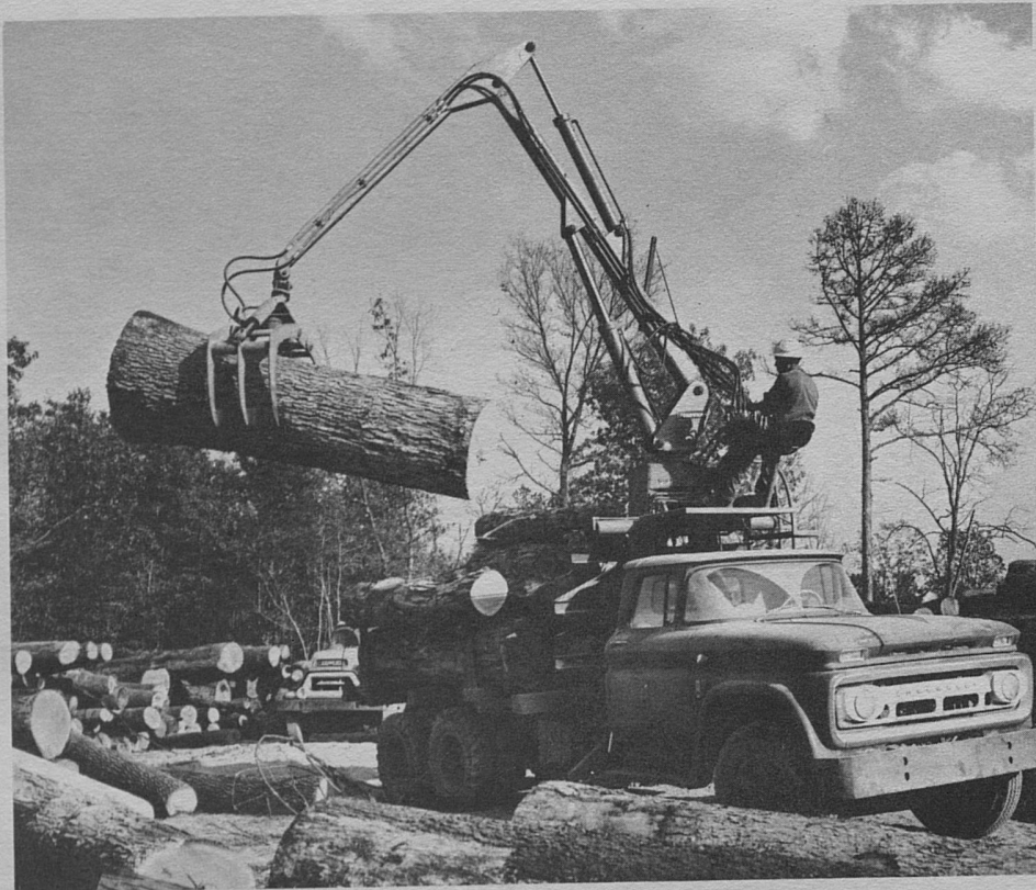
FIG. 3. -- MECHANICAL LOADERS PROVIDE A GREATER CAPACITY FOR HANDLING LOGS.
