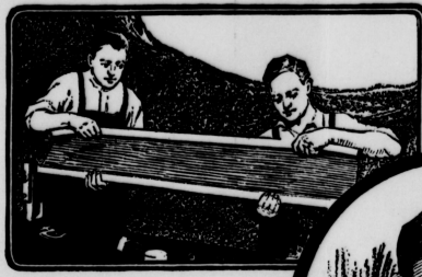
Winding high voltage insulation, 1894 — 2,500 Volts
