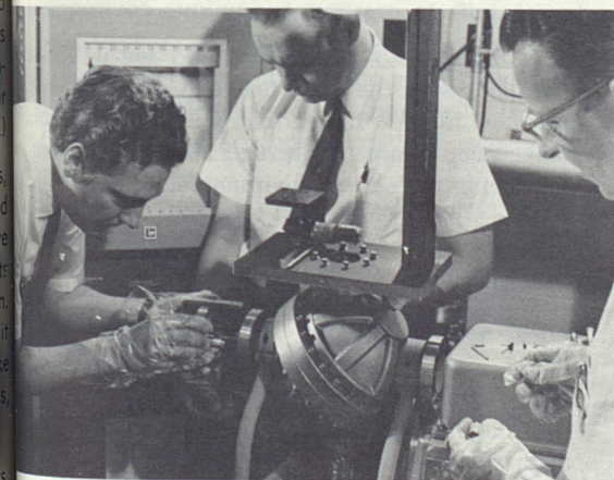
Researchers at the University of Kentucky College of Engineering bring place a sample of moon dust in an ultra-high vacuum study. Shown working with the vacuum system are, from left, Dr. Richard C. Birkebak, Jim Dawson, and E. B. Yates. The sample will be studied for its ability to transfer heat and to reflect light.
