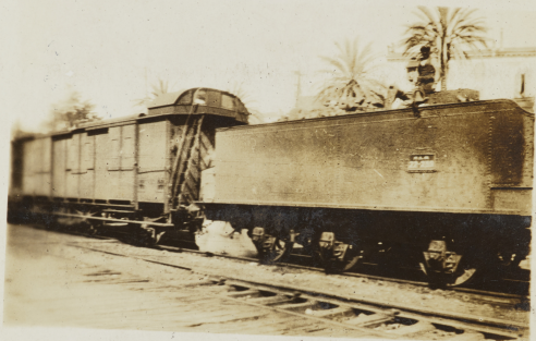
French Train, Tender and Caboose. Caboose on all trains both Fgt. and Passenger. Bell placed on Tender.
