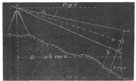
on whether x is an angle above or below the horizon, and on how high on the staff the middle line of sight reaches.
