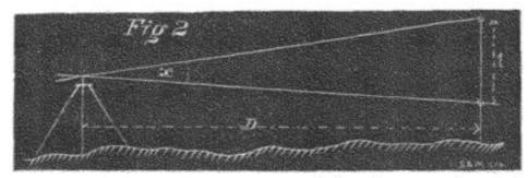
Now the angle is to be expressed by the number of screwthreads that are used in order to bring the telescope through the arc x; and from this one writes down tan x = c u, where c denotes a constant depending of the disposition of the instrument itself, and one obtains  $D = \frac{l}{tan x} = \frac{l}{cu}$ .
