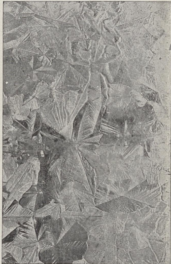
Figure 1. Shows a piece of new galvanized steel magnified only 12 times. Notice the elevations and depressions, showing the difficulty of cleaning. To germs they are as mountains and valleys are to us.
