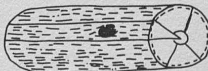
Any knot over two inches in diameter should be removed.
