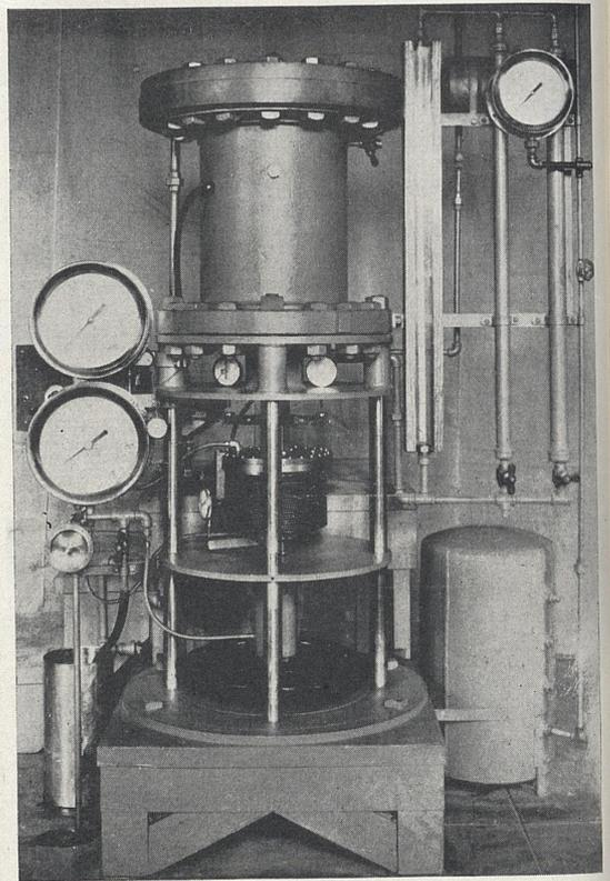
FIGURE 23.—STABILOMETER USED BY THE BUREAU OF RECLAMATION.
