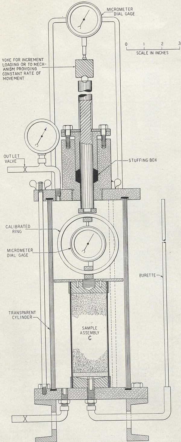
FIGURE 21.—STABILOMETER ASSEMBLY OF THE RING TYPE.
