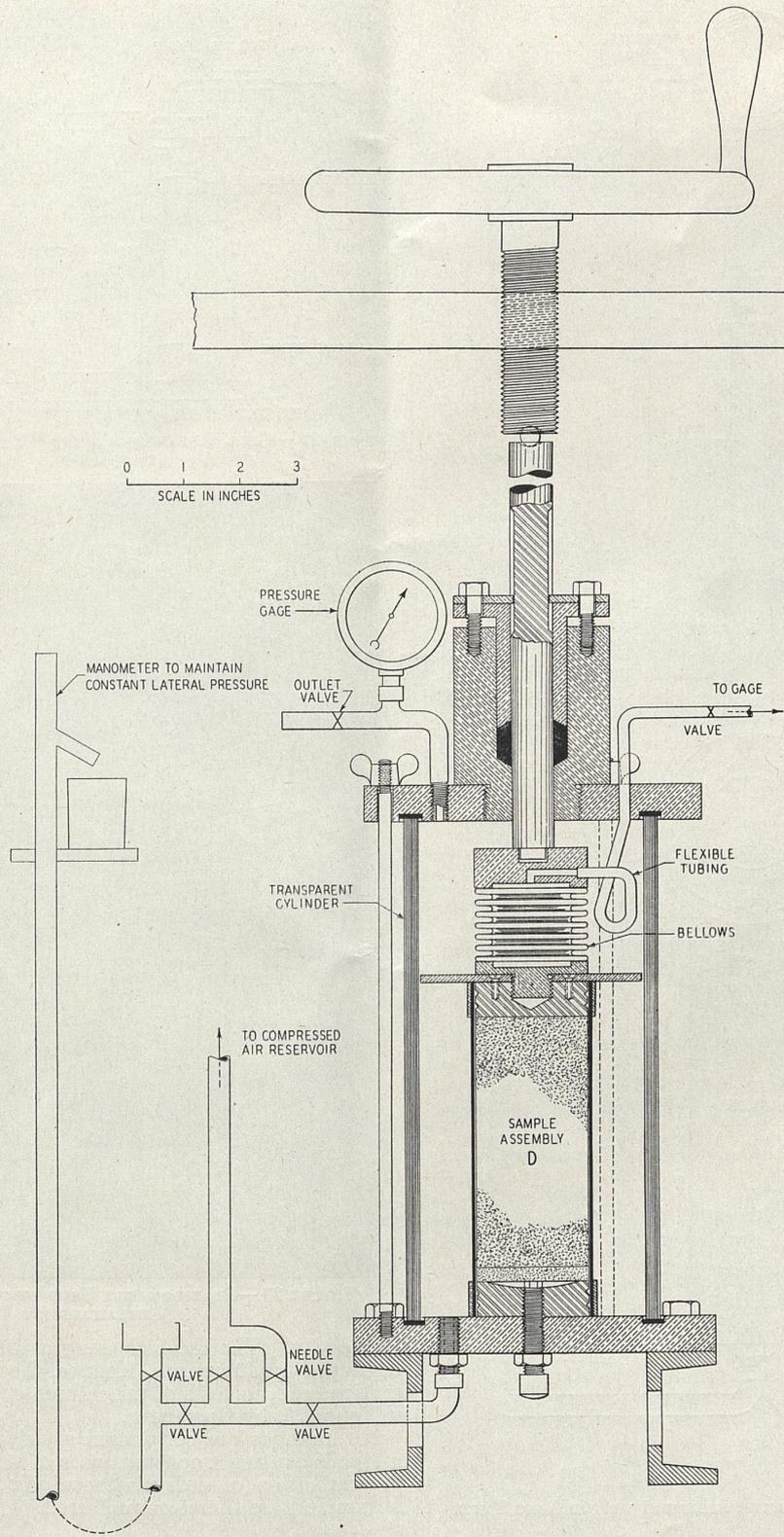
FIGURE 20.—STABILOMETER ASSEMBLY OF THE BELLOWS TYPE.
