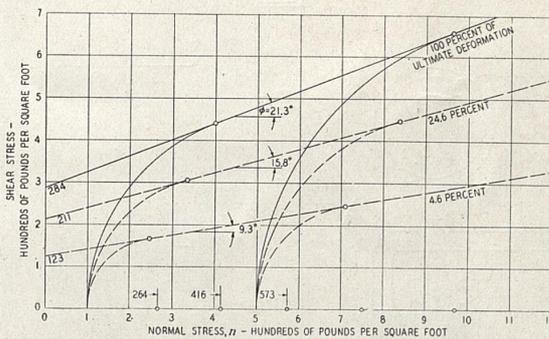
FIGURE 15.—GRAPHICAL ANALYSIS OF STRESSES IN CYLINDER.
