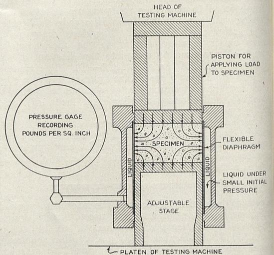
FIGURE 5.—DIAGRAM OF STABIOMETER DEVELOPED BY HVEEM.
