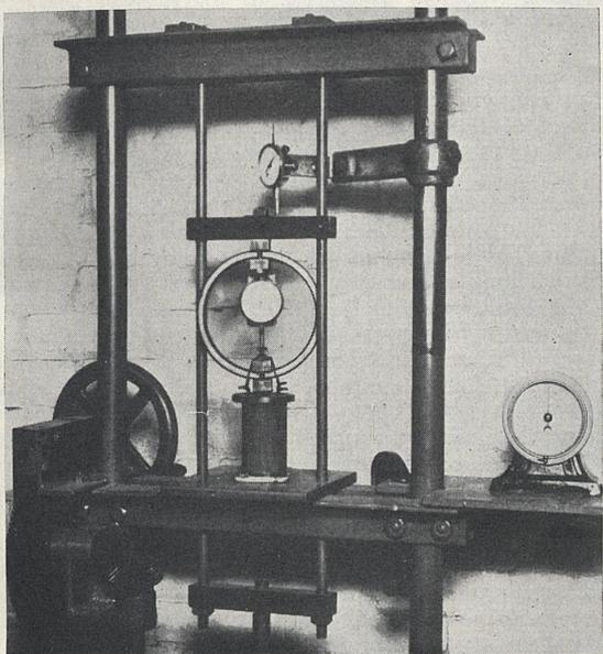
FIGURE 25.—LOAD MEASUREMENT BY CALIBRATED RING.
