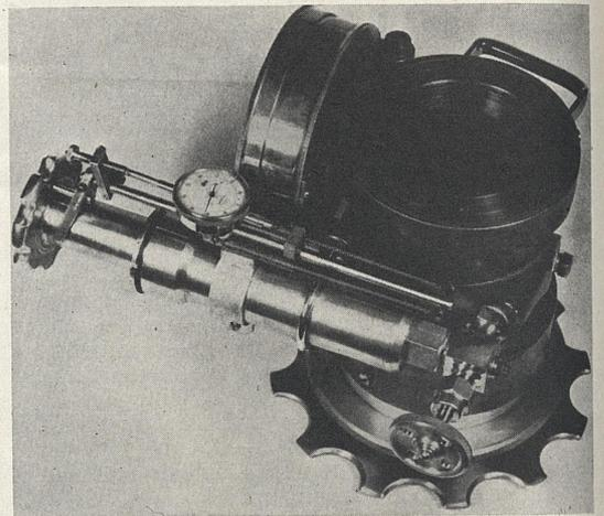
FIGURE 4.—STABIOMETER DEVELOPED BY HVEEM.
