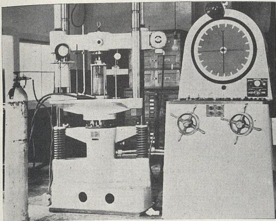
FIGURE 24.—APPARATUS USED IN MAKING TRIAXIAL SHEAR TEST AT HARVARD UNIVERSITY.
