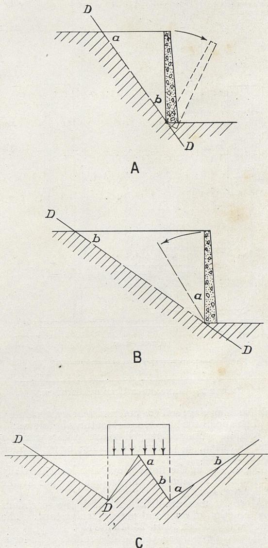
FIGURE 1.—SURFACES OF SLIP ILLUSTRATED.
