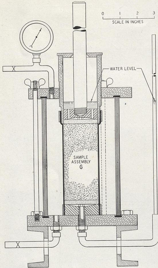
FIGURE 17.—STABILOMETER ASSEMBLY OF THE FIXED RUBBER TYPE.
