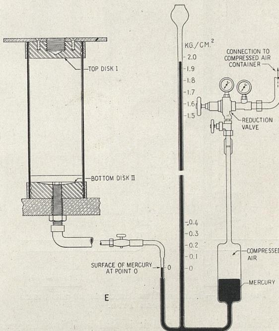
FIGURE 16.—STABILOMETER ASSEMBLY WITH SPECIAL MANOMETER.
