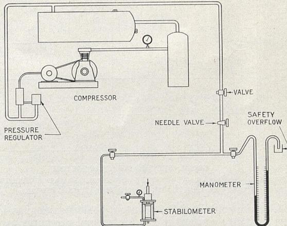
FIGURE 26.—STABILOMETER, MANOMETER, AND COMPRESSED AIR SYSTEM.
