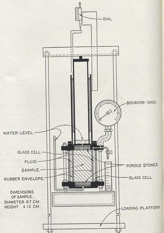
FIGURE 19.—CELL APPARATUS DEVELOPED BY THE DELFT LABORATORIES.
