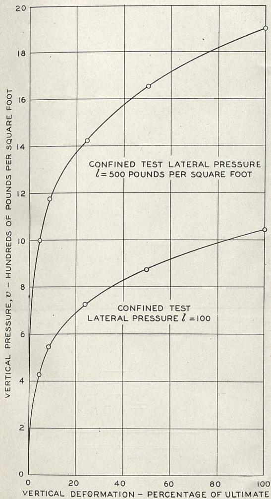
FIGURE 14.—STRESS-STRAIN RELATIONS FOR TWO SAMPLES.
