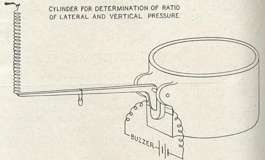
FIGURE 3.—APPARATUS DEVISED BY GOODRICH FOR DETERMINING RATIO OF LATERAL TO VERTICAL PRESSURES.
