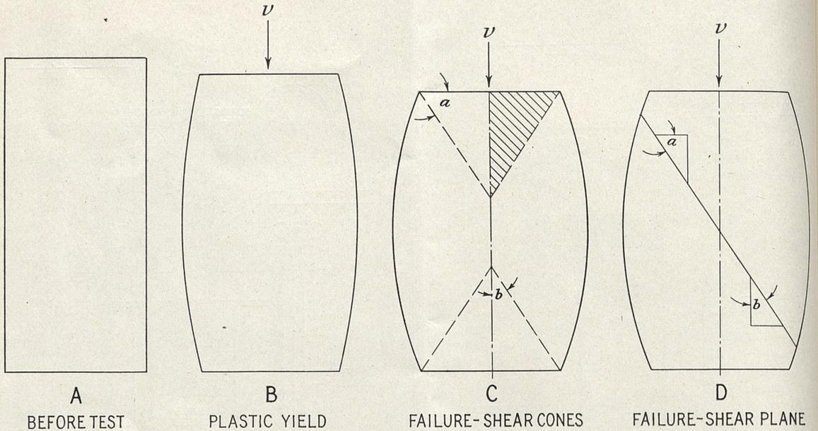
FIGURE 12.—DEFORMATION OF THE SAMPLE DURING TESTING.
