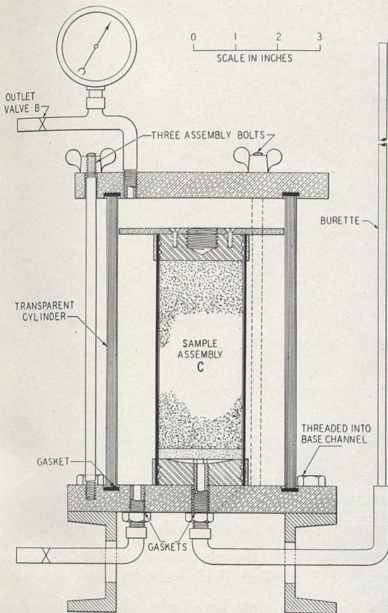
FIGURE 9.—PRESSURE CHAMBER FOR USE IN CONSOLIDATING SAMPLES.
