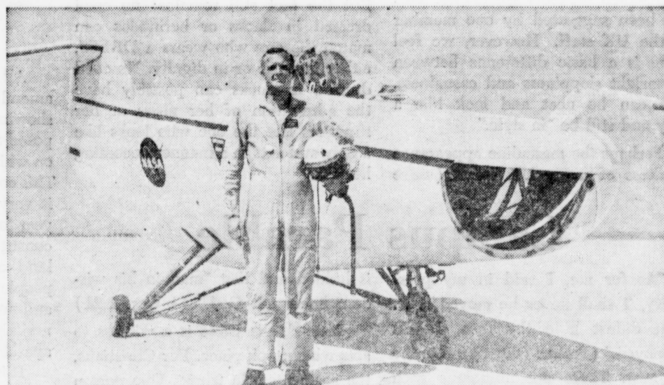
WINGLESS SPACE 'PLANE'—NASA pilot Milton Thompson stands in front of the M-2 lifting body, a wingless, maneuverable spacecraft capable of orbiting the Earth and landing airplane fashion. The craft is now being flight tested at NASA's Edwards Flight Research Center, Calif. Tests are aimed at finding a vehicle to ferry astronauts back from space missions.
