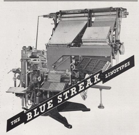
**74 features** that contribute to efficiency of operation... ease of maintenance... improved appearance; including the Optic-Aid Front which increases production by eliminating distracting motion and reflections in front of the operator's eyes, and the One Turn Shift.
