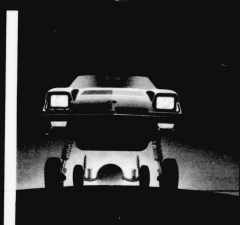
Four-wheel independent suspension.
