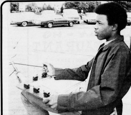
Kenneth Elliot, an employee for Neighborhood Youth Corps, counts the number of cars passing through an intersection. This information will be used to regulate traffic lights.
