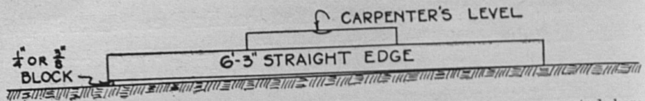
Fig. 4. A straightedge and carpenter's level used as suggested here will help in making an even grade. A \frac{1}{4} " block gives a grade of 4" per 100 ft. and a \frac{3}{8} " block a grade of 6" per 100 ft.
