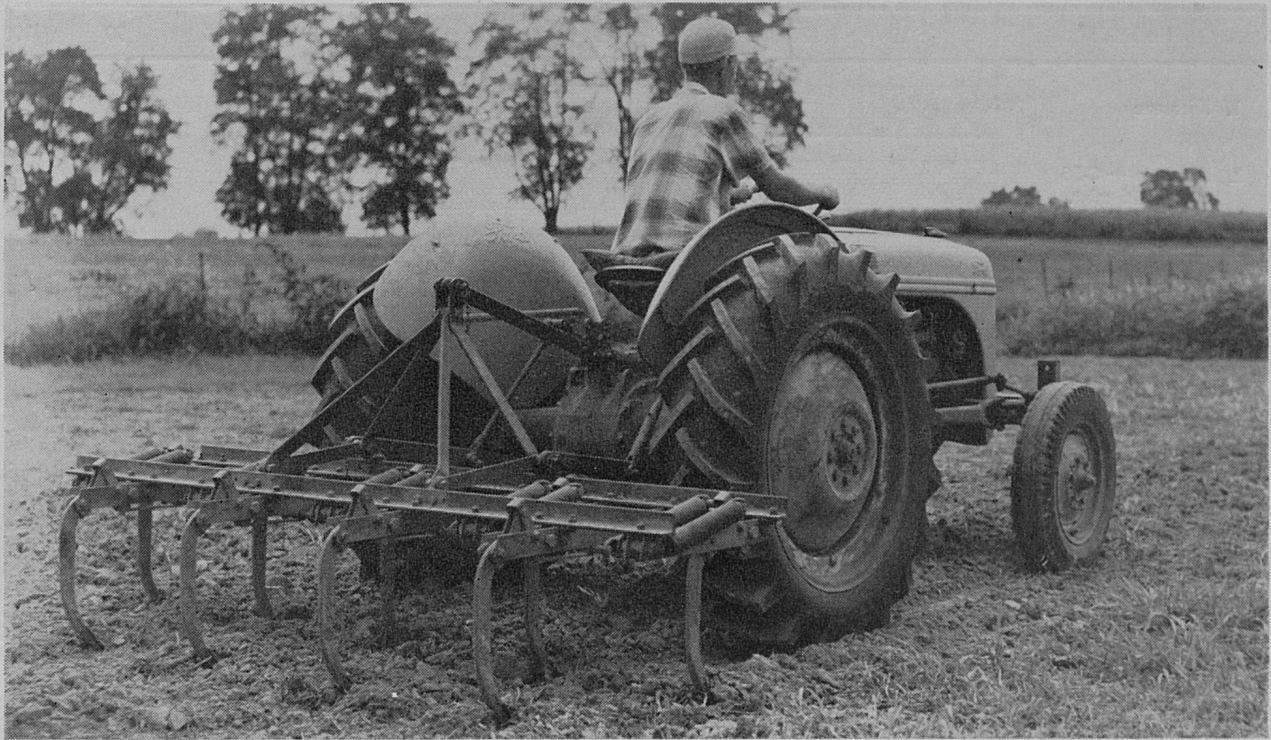
Clean cultivation every two weeks during summer after breaking Johnson grass land is a good method of controlling rootstocks in dry summers. A field cultivator equipped with overlapping flat sweeps is best for such cultivations, but a disk harrow is satisfactory.
