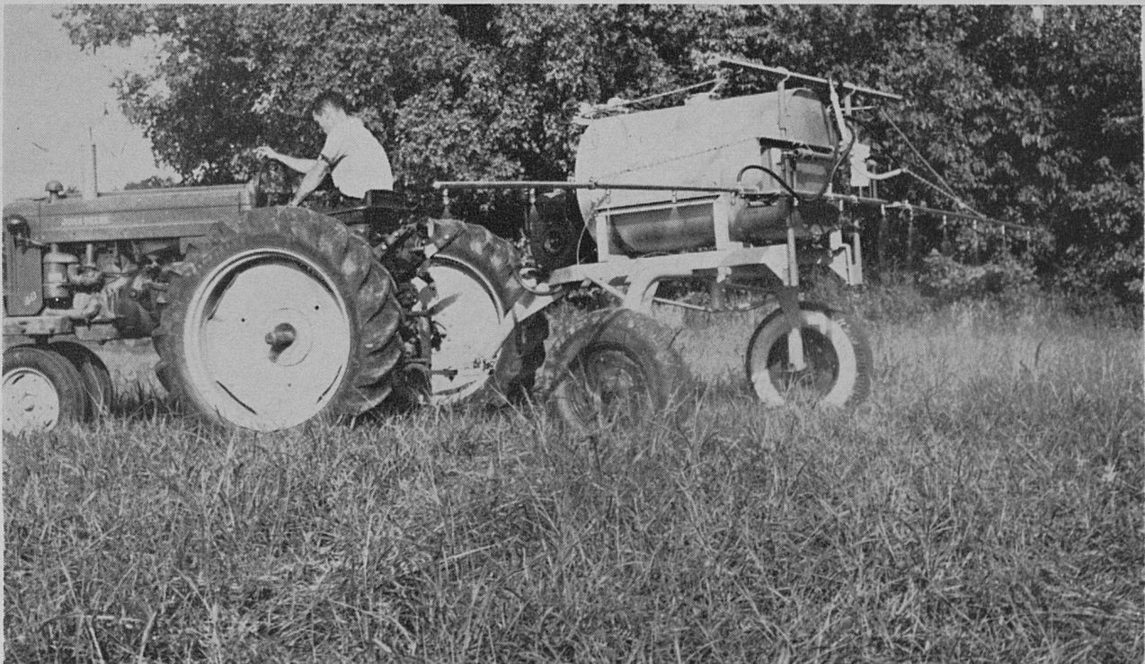
Spraying short Johnson grass with dalapon solution. Boom-type sprayers give a desired uniform coverage of the plants.
