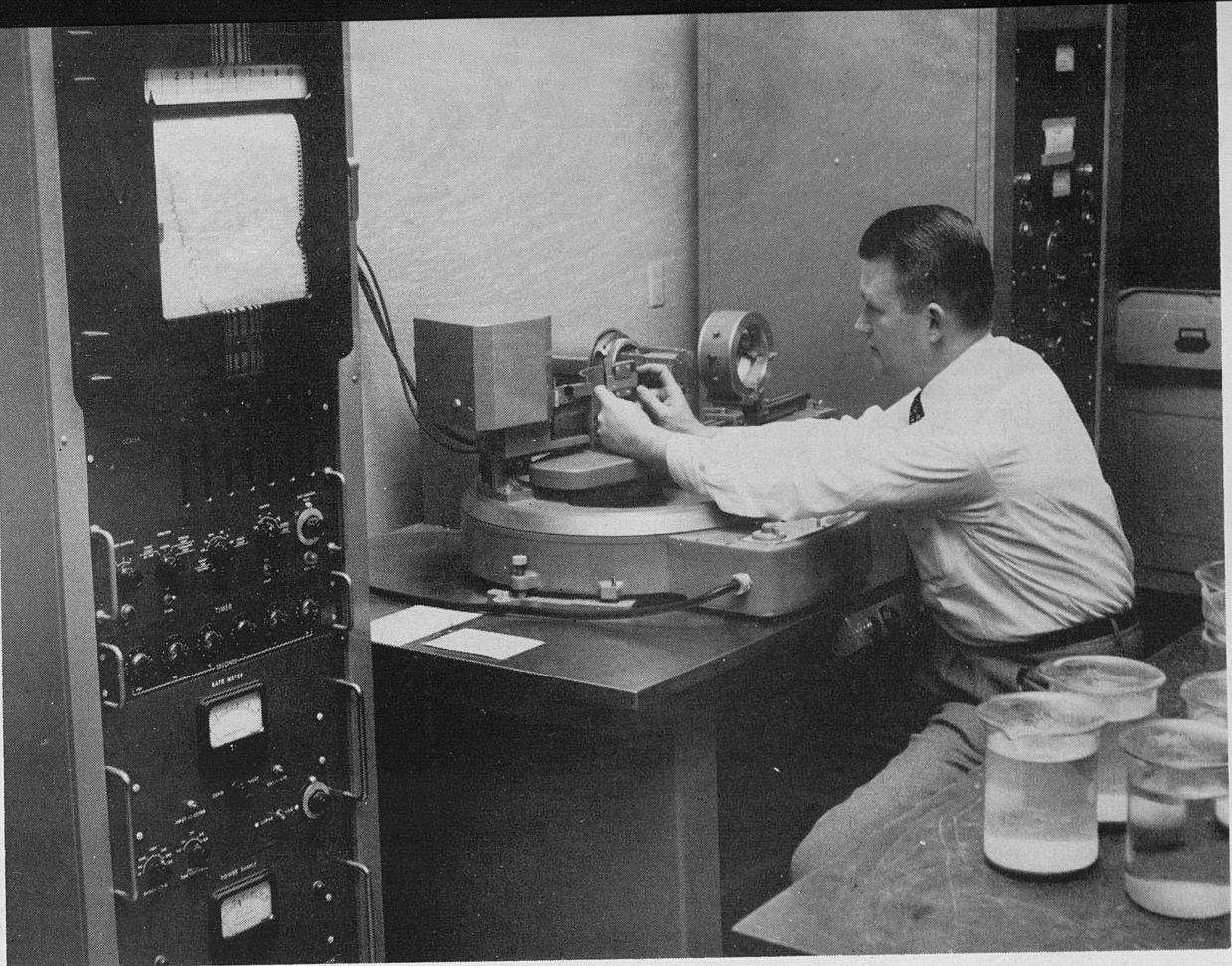
(Above) In making an X-ray examination of the mineral matter in a soil sample, a small portion is put on a glass slide which, in turn, is placed in the path of an X-ray beam. After the beam encounters the mineral matter the pattern is recorded by the equipment in the foreground. Behind and to right of the author is the X-ray generator.
