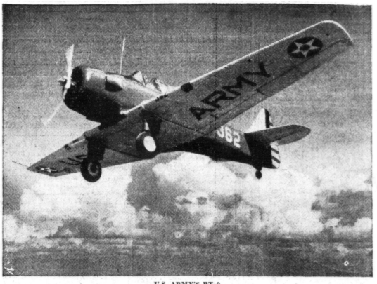
Powerful with 400 horse-power engines and capable of speeds up to 170 miles per hour, sleek trainers like this one are flown by Army Air Corps cadets in primary training.
