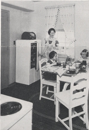
Planning for safety in dwelling-unit design. Note that range is placed across the room from the window to prevent possibility of curtains catching on fire.
