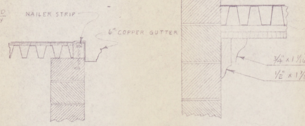
SECTION "E-E" SHEET 6 GUTTER DETAIL Scale: 3/4" = 1'-0"
