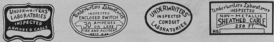
FIGURE 2. Labels that should be found on wiring equipment, indicating that the materials conform to the minimum requirements of the Underwriters Laboratories. They do not specify the exact quality of the product.
