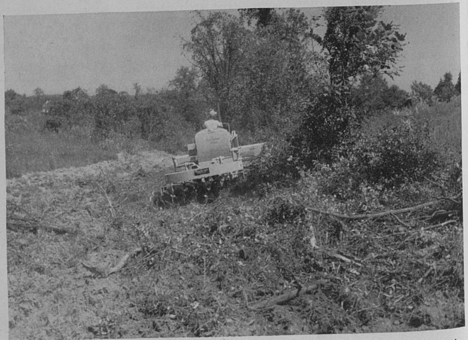
Or the bushes and smaller trees may be chopped up and worked into the soil by a bog harrow.
