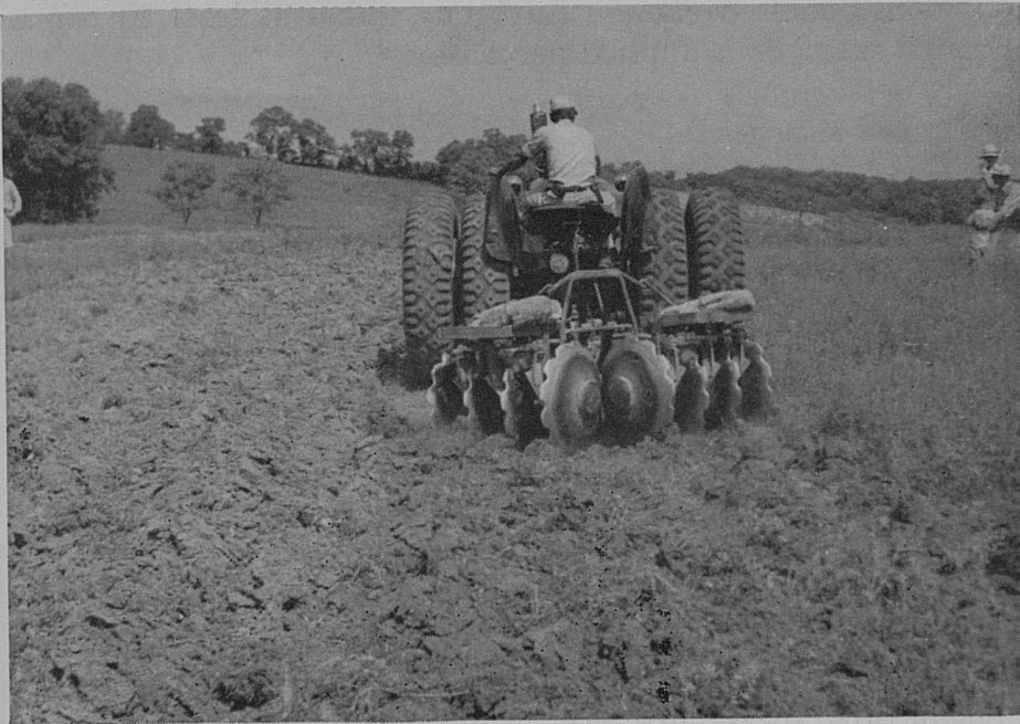
The bush or bog harrow is popular in Kentucky for preparing a seedbed on old pastures on sloping land because it works the vegetation into the soil and offers less exposure to erosion than on land that is plowed.
