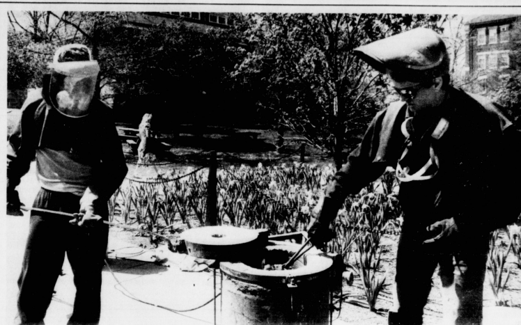
Some like it hot. Two UK students make an aluminum cast using the Styrofoam burnout process Friday. The demonstration was part of the College of Fine Arts' week-long Arts Festival.
