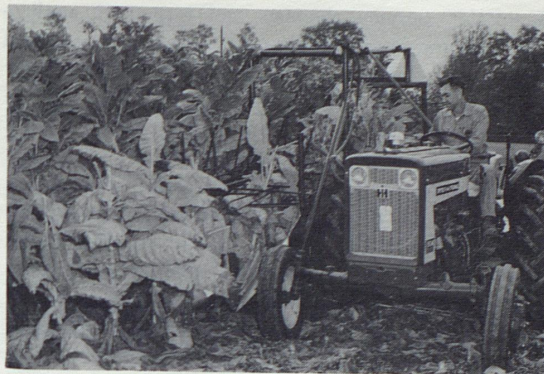
Agricultural engineers are developing a tobacco harvester in an effort to speed up harvesting and reduce the labor involved.
