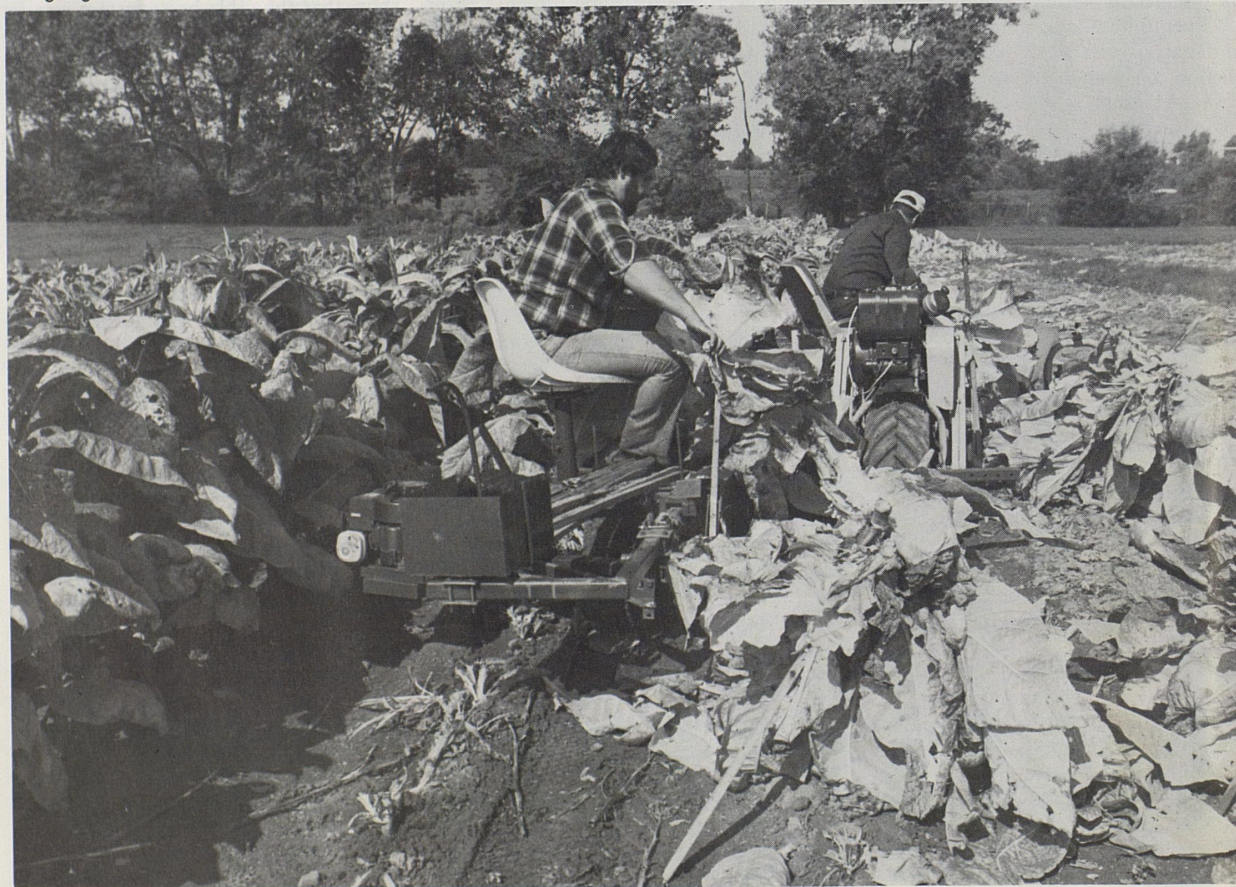
UK ag engineers use an attachment on a one-row harvester to cut two rows of burley at the same time.
